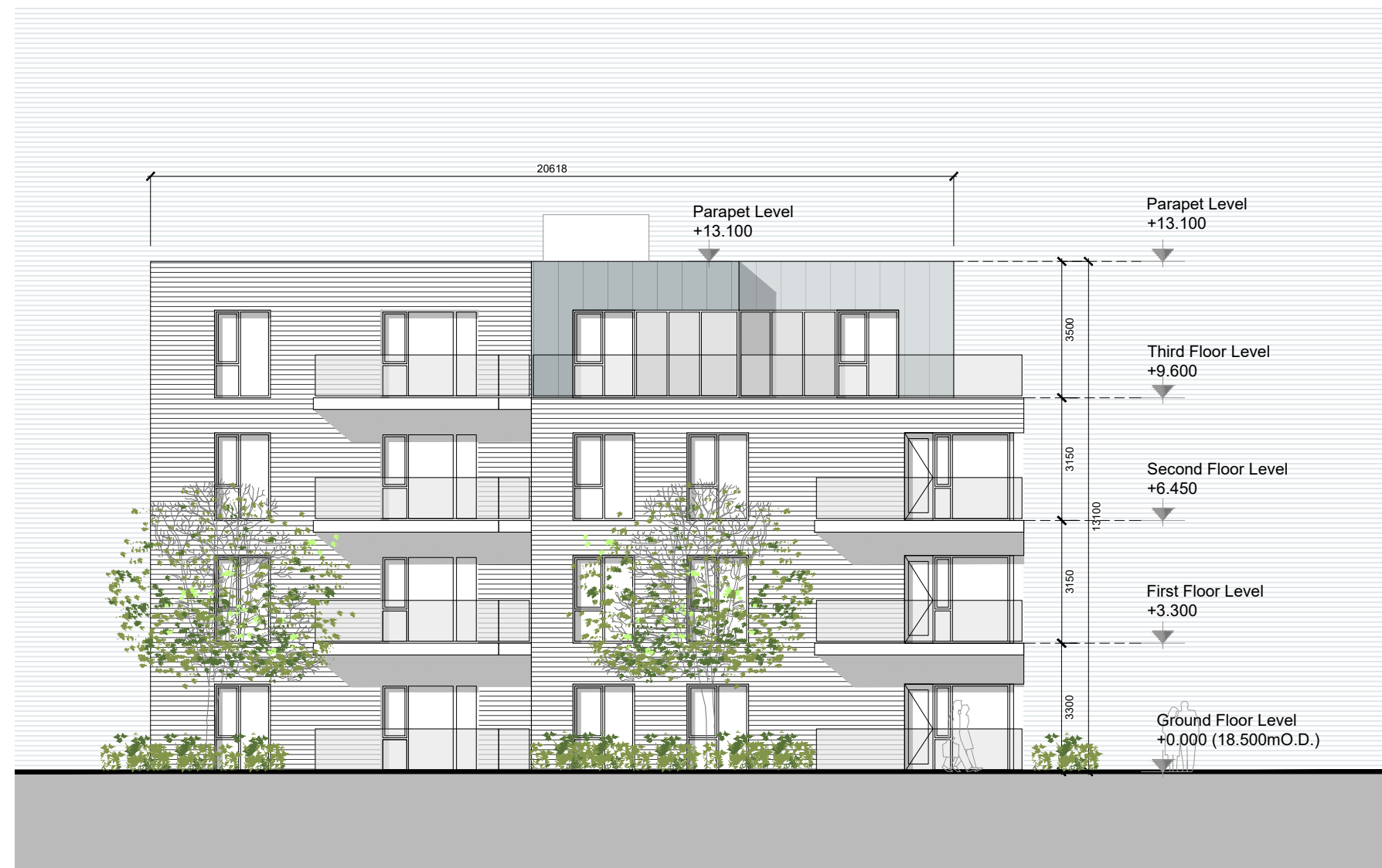
South Facing Elevation AA Character Area 3 (Red Stock Brick)
